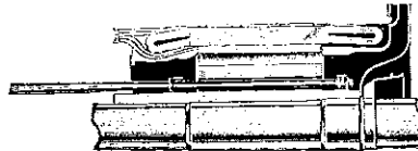
Shaft and Commutator Removed
