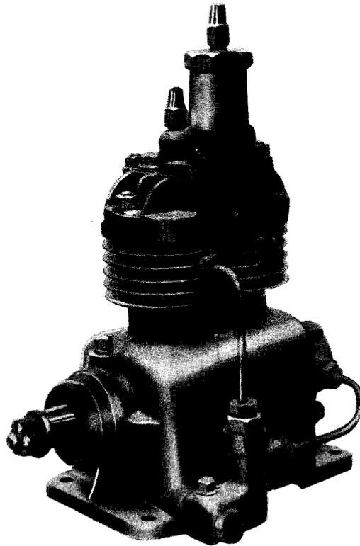
This compressor has automatic inlet (1) and delivery valves (2) of the poppet type, one pair for each cylinder, located in the cylinder head (3). The valves are assisted in their action by light springs (4).
