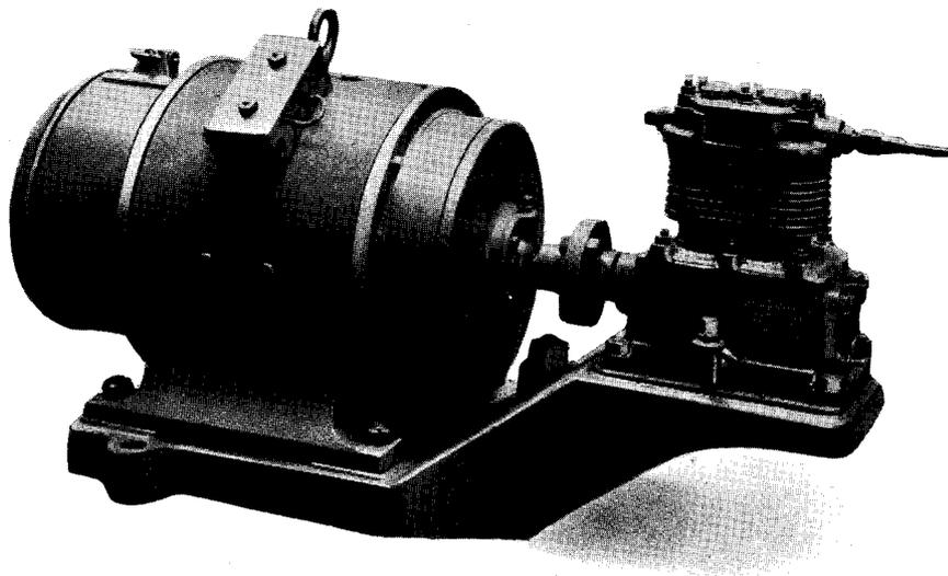
Type O.35 Compressor, coupled to  $\frac{1}{2}$  h.p. 500-volt Motor.
