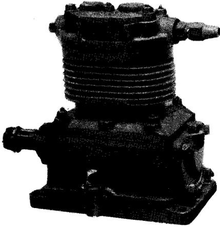
This compressor is similar in many respects to the type M. 50, but is not fitted with the pressure regulator or the automatic oil pump.
